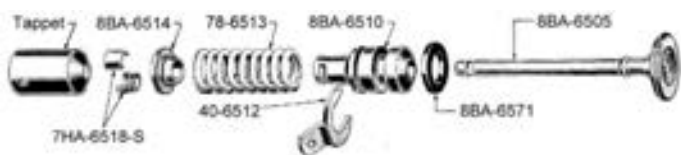
Valve With Solid Guides
